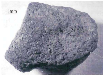
A typical black and highly porous polycrystalline carbonado-diamond (5.3carats) from Bahia, Brazil
